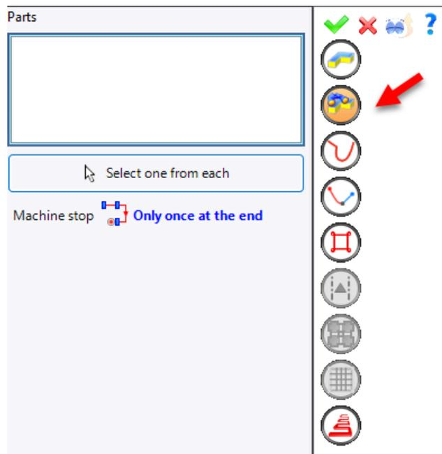
Parts can be selected individually or via the **Select one from each** button, which automatically picks one part of each type. A stop is applied either after machining each prototype part or upon completion of all prototype parts.
