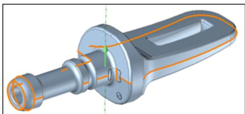
*Example of searching for candidate edges in **Precision** mode. A closed path cannot be created due to the selection of unnecessary edges.*
