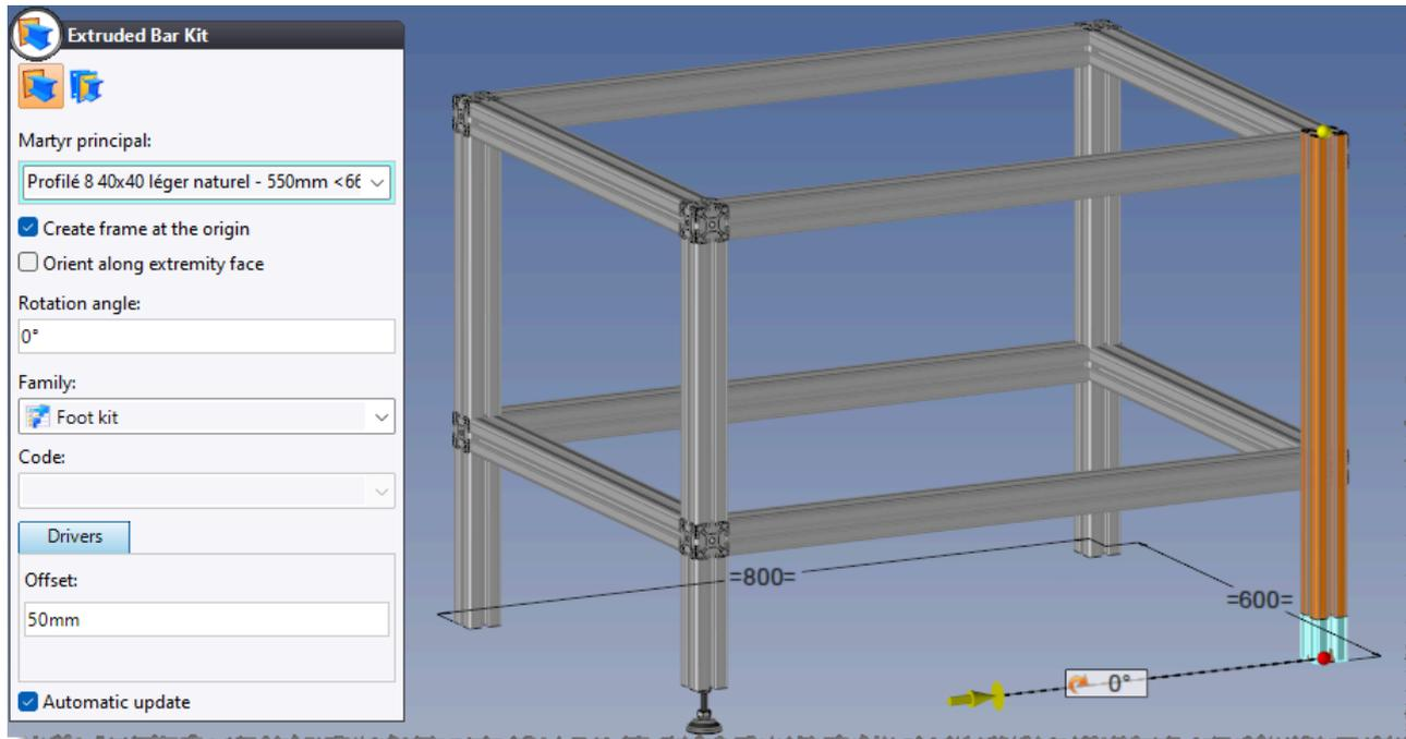
Example of positioning an extruded bar kit at the end of an extruded bar.
