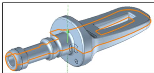
*The **Isoclines** option automatically imprints the missing silhouette curves along the outer contours, ensuring the creation of a closed path.*
