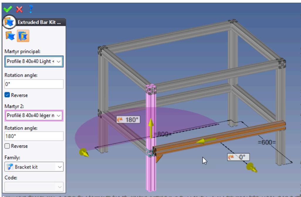
Example of positioning an extruded bar kit at the intersection of two extruded bars.
