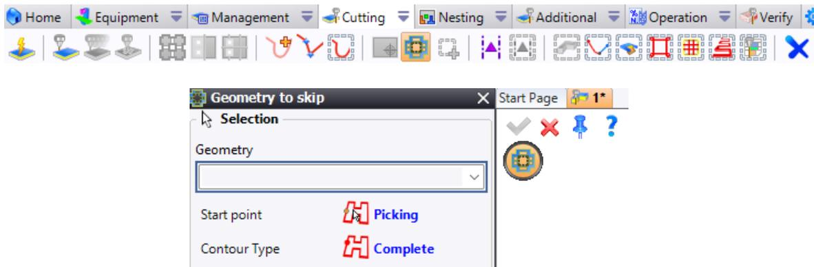
By default, ignored geometry is represented by black dotted lines, but the color can be customized via **Tools > Options > CAM Options > Sheet Metal Cam Options > Machining Attributes**.
