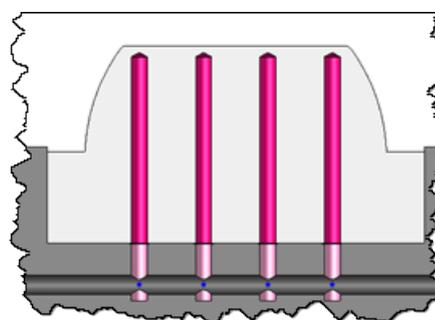
*The lengths of the two holes are defined by the cooling style.*
