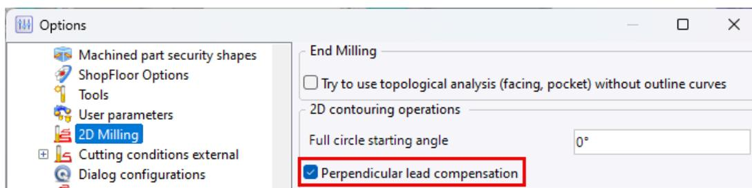
It can force or not the perpendicular lead compensation on the first movement.
