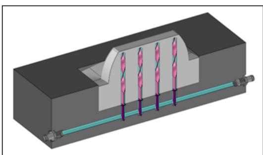
*Two self-locking baffles are automatically added when creating baffle lines.*
