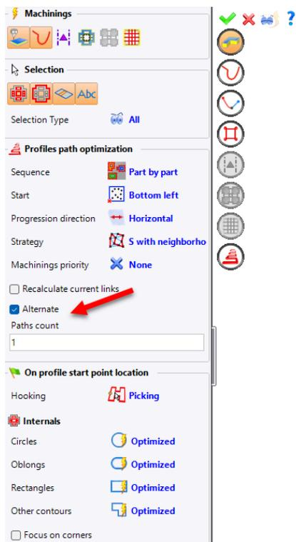
The tool path alternates between machining passes and skipping an equal number of operations, as specified, to prevent overheating the same zone.
