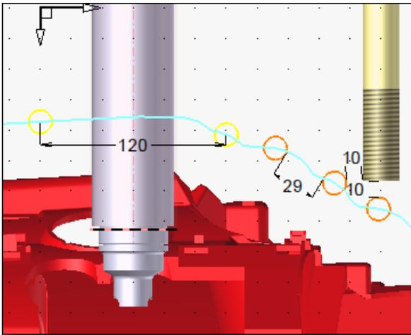
*Version 7.18: The interval between the yellow hole and the first orange hole was significantly smaller than the interval between the following 29mm holes.*
