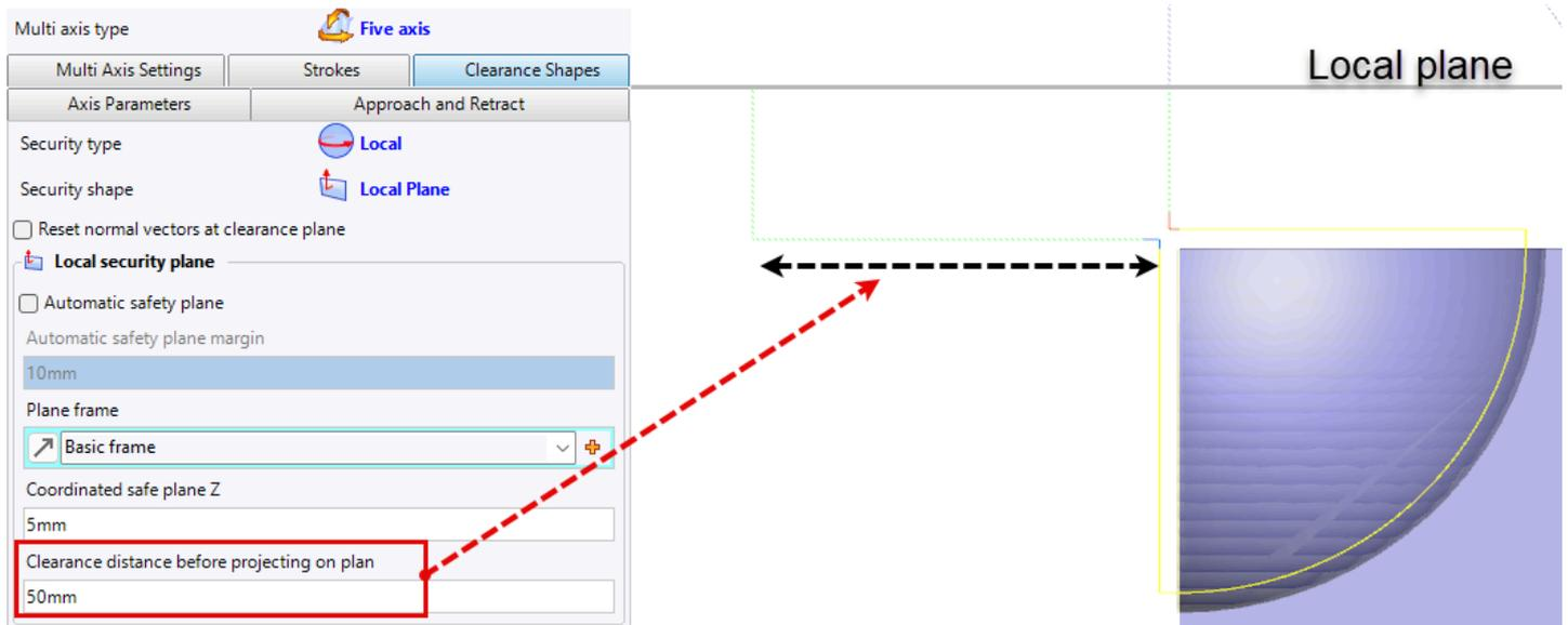
If the local safety plane is still not reached beyond the specified clearance distance, a perpendicular projection is made to determine the shortest path.
