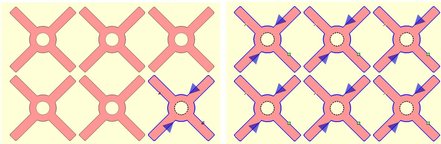
*In this example, the machining operations have been propagated from the bottom right-hand part to all identical parts.*
