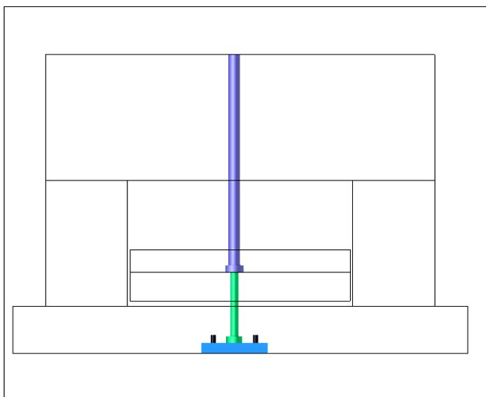
*Example of a method including a cylindrical pin and a tubular pin, with a precision plate.*
