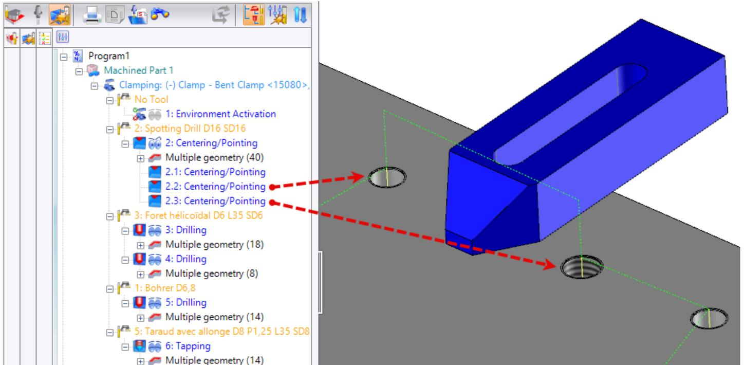
*The link between two holes from different operations correctly avoids the fixture.*
