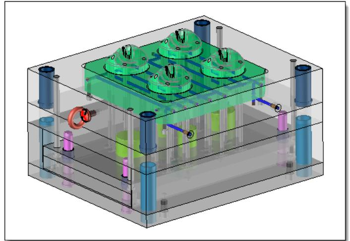
*Once the circuit is created, it can be adjusted to add any missing drillings.*
