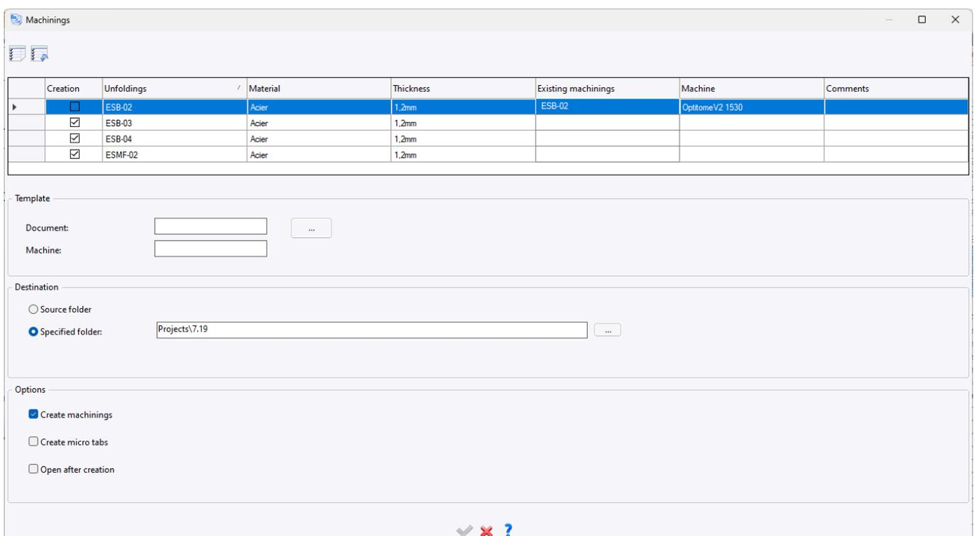
*In the example above, three sheet metal machining operations will be created as machining already exists for the first unfolded part.*
