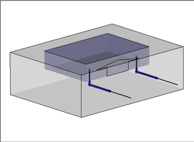
*The method automatically generates the cooling circuit between two parts.*
