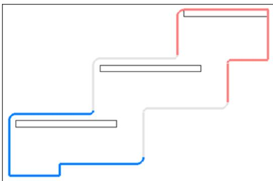
*Sawtooth stringer type document template It is defined by three sketches representing each part of the stair flight (start, intermediate and end of the flight).*
