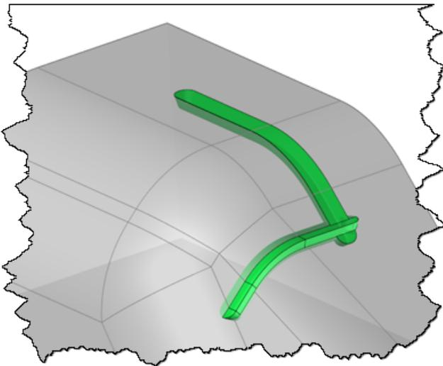
*Previously, the sections were oriented by the mold opening direction, sometimes limiting the precise positioning of the circuit.*
