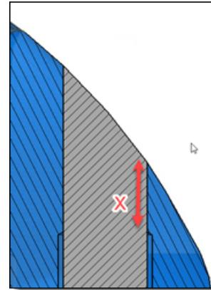
*Boring length computed from the minimum machined length.*
