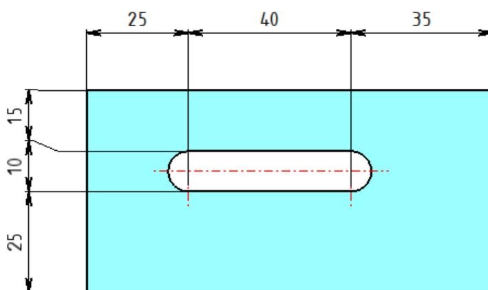
*In the above example, the detection of the extremities of the horizontal and vertical lines automatically dimensions the oblong hole.*
