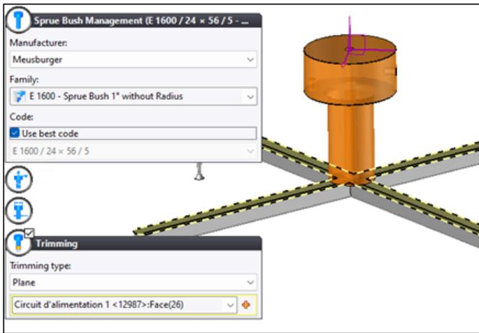
*Sprue bush sizing and limitation with the new **Sprue Bush** command.*
