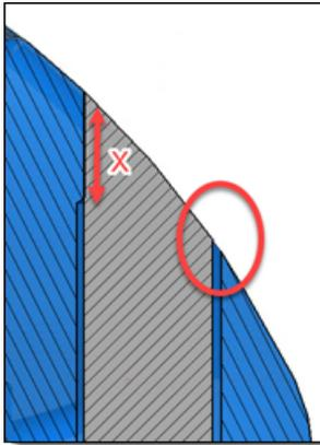
*Boring length computed from the machined length.*
