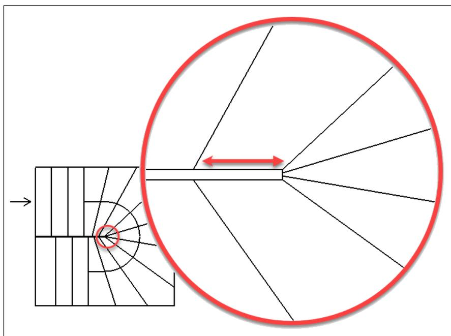
*The minimum collar is only applied to the flight permitting.*
