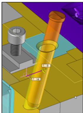
*Angle pin process with chamfer-type blend.*
