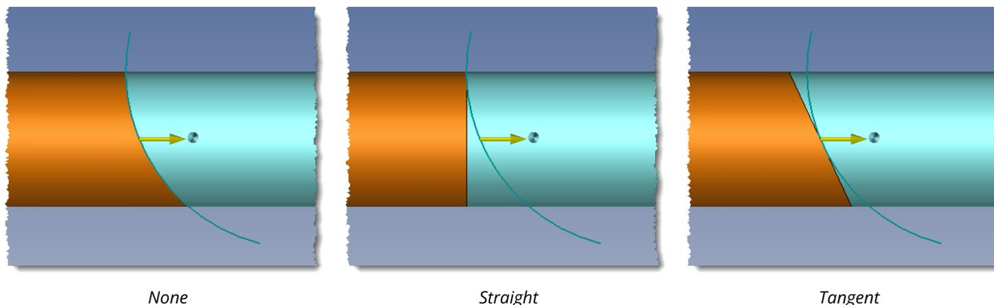
Extruded bars imported and converted via the **Modeling > Sheet Metals Recognition** command are now supported by extruded bar trimming commands.
