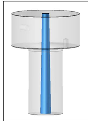
*The runner shape is automatically limited with the sprue bush.*
