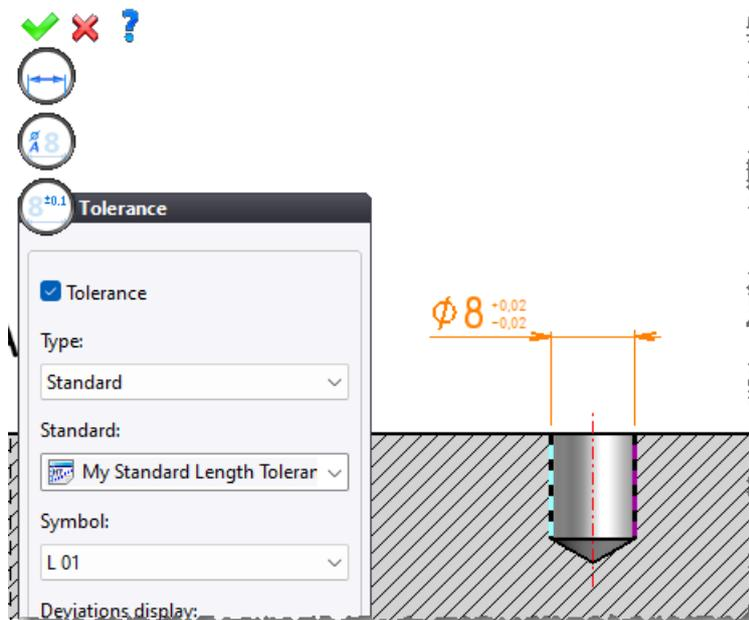
*Use of dimensional tolerance standard in dimensioning.*
