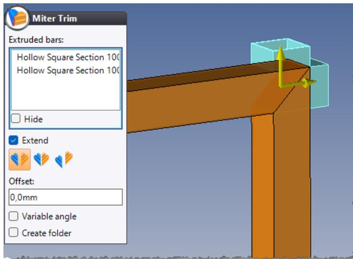
The **Variable angle** option has been replaced by five icons to manage trims between complex extruded bars.
